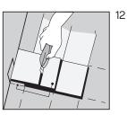
The last and first plank can be cut in the correct width. Place the last plank on top the second to last plank. Mark the plank with the help of a piece of plank without locking the strip
