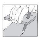
Transfer the shape of the wall to the planks. Do not forget to allow 5mm(0.2") for the expansion gap.
