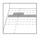
Measure the room accurately, at right angle to the direction of the planks. The planks in the final row should be at least 5cm (2") wide If necessary, the planks in the first row can be cut to a smaller size.
