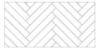
Chevron: There are left and right planks/elements which are alternately located in the package. A stainless cutting rail/steel strip will help you to put on the first row. Care must be taken to ensure that this is exactly in place and direction.
