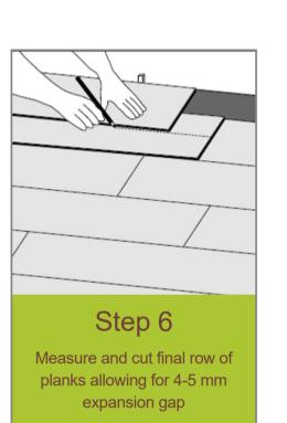
Step 6 – Measure and cut final row of planks allowing for 4-5 mm expansion gap
