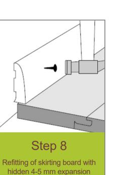
Step 8 - Refitting of skirting board with hidden 4-5 mm expansion gap
