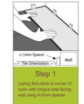
Step 1 – laying of first plank with tongue side facing wall using 4-5 mm spacers
