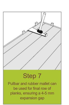
Step 7 – Pullbar and rubber mallet can be used for final row of planks, ensuring a 4-5 mm expansion gap
