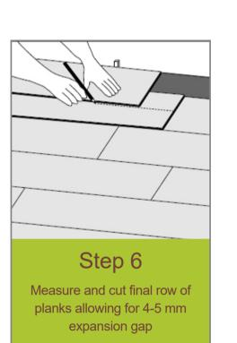
Step 6 – Measure and cut final row of planks allowing for 4-5 mm expansion gap
