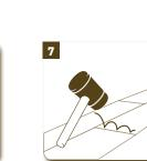
Hammer the planks together, beginning with the small side. Hammer taps must be close to one another to ensure that planks are firmly locked together.
