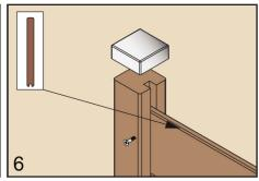
As the top plank, you can use the finishing board without the upper spring. After putting on the enclosed cover cap, you have finished the construction.
