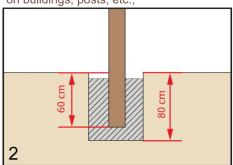
Fill the holes with concrete. Pay attention to the corresponding curing times of the concrete manufacturer.
