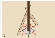
The post must be aligned at right angles from all sides. Fix it with an auxiliary construction.
