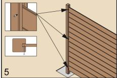
Three screw connections through the post into the plank, provide sufficient support and stability.
