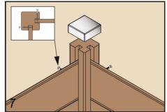
When screwing the corner posts, please note that the screws should be placed from the outside.
