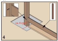
As a constructive wood protection, we recommend a distance of approx. 4 cm to the substrate to protect the material from possible weather damage.
